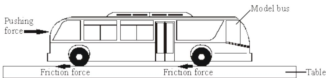
(i) At first the pushing force does **not** make the model bus move. Explain why.
