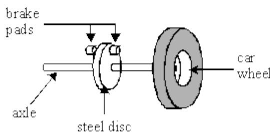
The force of friction between the brake pads and the steel discs gradually stops the car.
