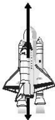
Weight of shuttle, fuel tanks and booster rockets plus air resistance
