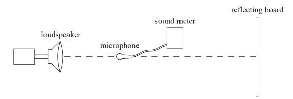
A loudspeaker is placed at a distance from a vertical reflecting board. Sound waves reflect off the board and set up a standing wave between the loudspeaker and the board. A microphone connected to a sound meter is moved in a straight line from the loudspeaker to the board. As the microphone is moved, the sound meter records the varying intensity of the standing wave.
