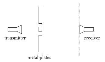
As the receiver is moved along the dotted line, alternate points of maximum and minimum intensity are detected.
