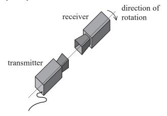
The receiver is rotated through 180° relative to the transmitter.
