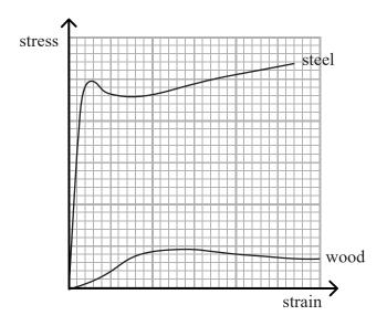
Discuss how the use of steel, rather than wood, has made the construction of faster and taller roller coasters possible.
